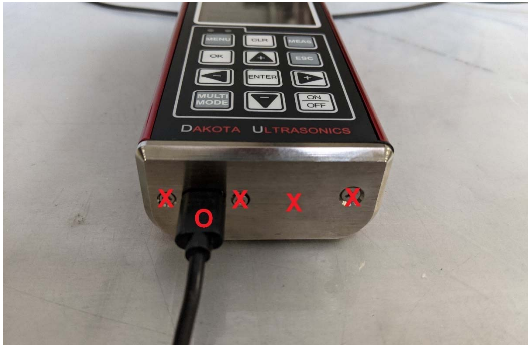
Figure 10. Electrostatic Discharge, Bottom of EUT Test Point
