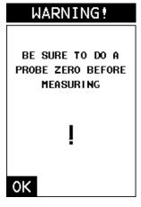
**Note:** The probe zero disk (battery cap) is located on the top end cap of the gauge. The warning screen will be displayed following the selection and overwrite of a new transducer.
