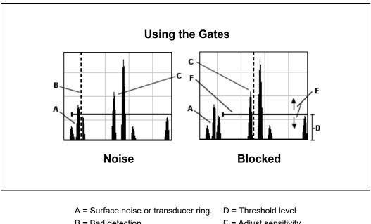
B = Bad detectionE = Adjust sensitivityC = Good detectionF = Gate
