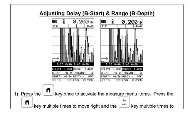
**Note:** The **Delay (B-Start)** and **Range (B-Depth)** are also used to adjust the parameters of **Scan Bar**.
