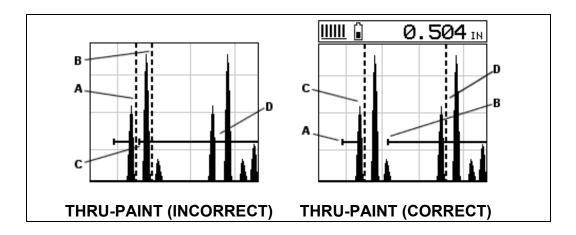
Refer to the 'incorrect' diagram above. Point (A) represents the detection on the first back wall echo, indicated by the broken dotted vertical line. The actual second back wall reflection should be detecting at point (D). However, the hold-off (C) is setup incorrectly and the *MX2-DL* is detecting the ring down noise of the transducer on the first reflection, rather than the actual second back wall reflection shown at (D).
