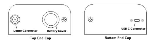
The top & bottom end panels are where all connections are made to the *PZX1-DL*. The diagram above shows the layout and description of the connectors:
