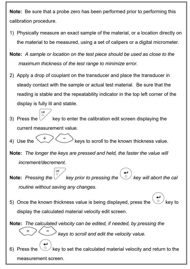
Note: CHECK YOUR CALIBRATION! Place the transducer back on the
