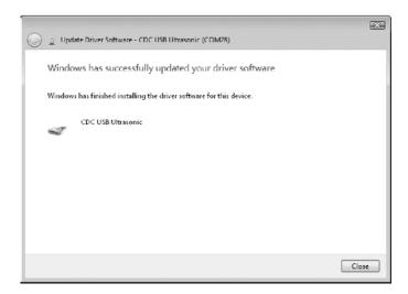
Open device manager again to reference the communications port assigned to the CDC device, it will be displayed to the right of the CDC device. Now that the driver has been successfully installed, a 'keyboard wedge' with serial communications capability can be used to connect to the ZX-6 and will capture the measurements to your PC when the ENTER key is pressed:
