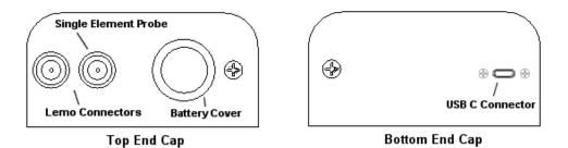
The top & bottom end panels are where all connections are made to the **ZX6-DL**. The diagram above shows the layout and description of the connectors:
