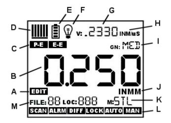
The **ZX6-DL** uses a custom glass LCD backlit low temperature display for use in a variety of climate conditions. It contains graphic icons, as well as both 7 and 14 segment display areas. Let's take a closer look and what all these things are telling us:
